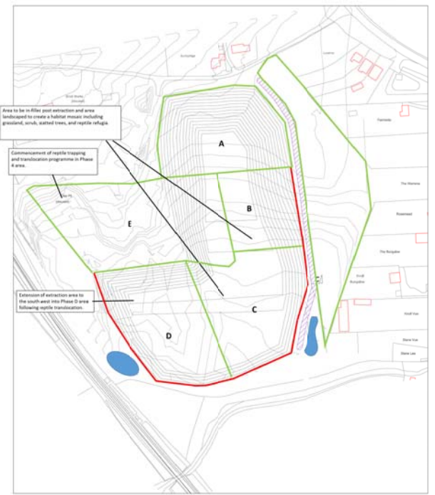
PHASE 3 - WIDENING QUARRY TO WEST
