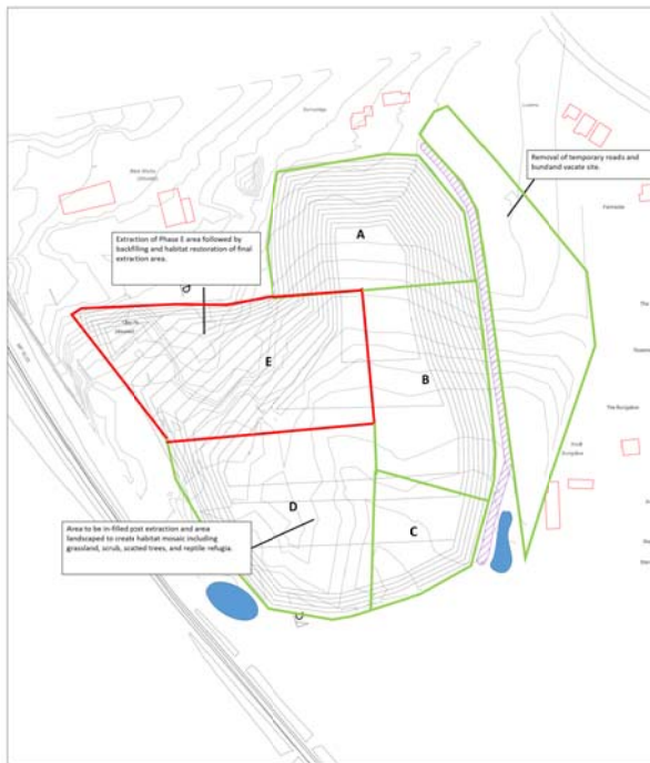
PHASE 4 - EXTRACTION PROGRESSING TO THE WEST TO COMPLETE EXCAVATION
